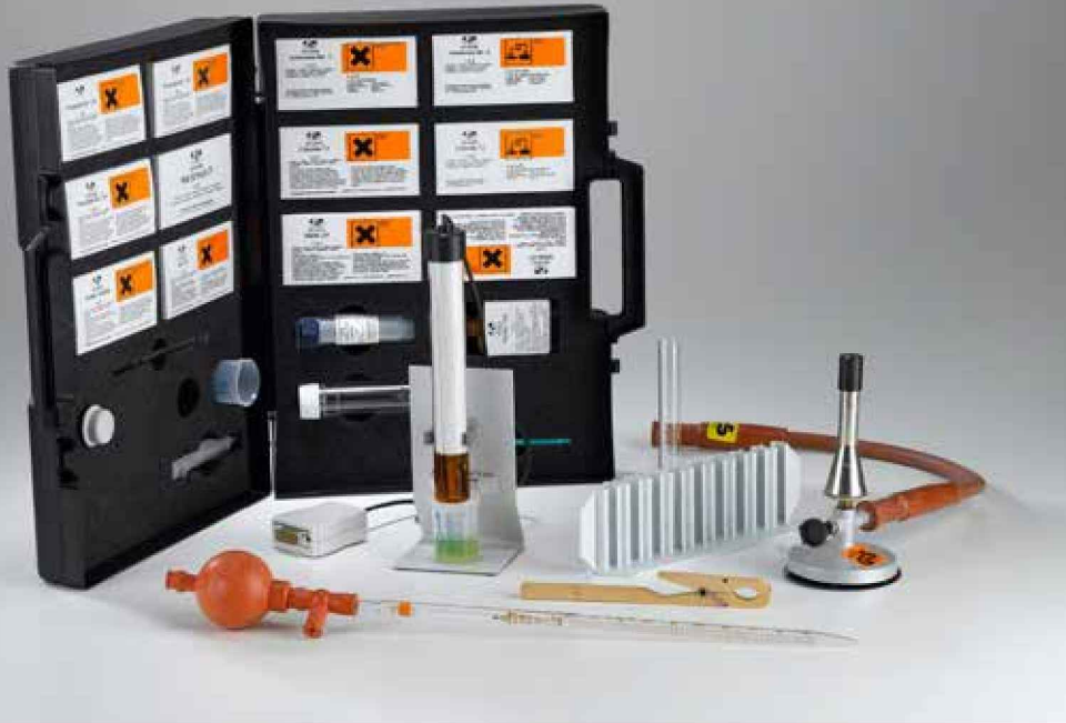
Determination of water contents with indicator reagents and immersion photometer (C3.6.1.1)
